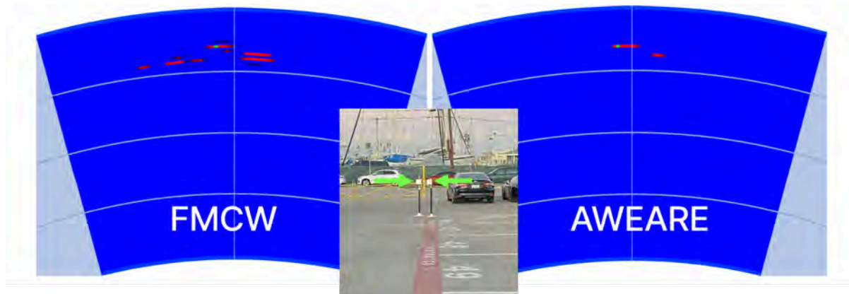
Figure: FMCW radar viewing two adjacent radar targets sees ghosts; AWEARE eliminates these ghosts. Both images were taken with identical hardware at the same filter settings.
